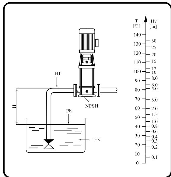
Check and ensure that the pump is not at cavitation state.
