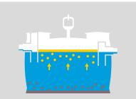
Grease and oil rise to the top and form a grease layer that is retained between the inlet and outlet.
