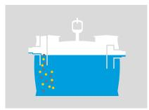
The contaminated wastewater is routed into the grease separator where it is slowed down by a deflector plate.
