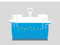
Substances that are heavier than water sink to the bottom and settle in the sludge trap.
