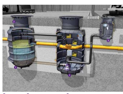
1 Grease separator 2 Height adjustable upper section 3 Disposal chamber
